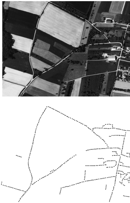
Fig. 4. Aerial image © IGN (top) and extracted road network, the links represents interactions between points of the solution (bottom).
