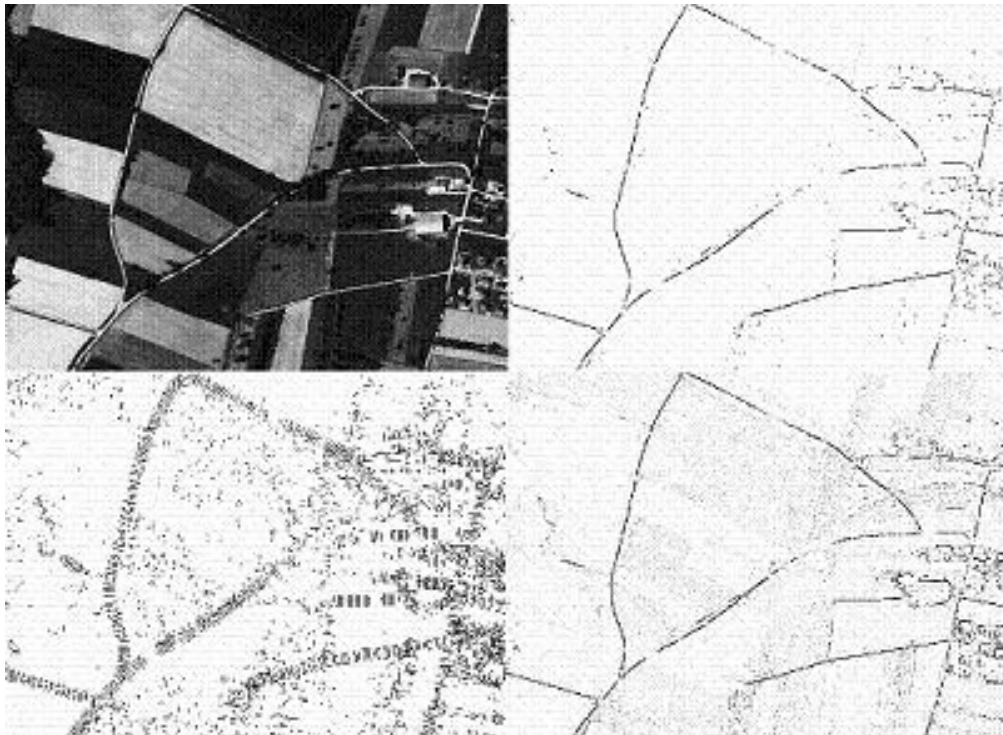
Fig.1. Aerial image © IGN (top left), contrast filter (top right), local orientation (bottom left) and LRD (bottom right).
